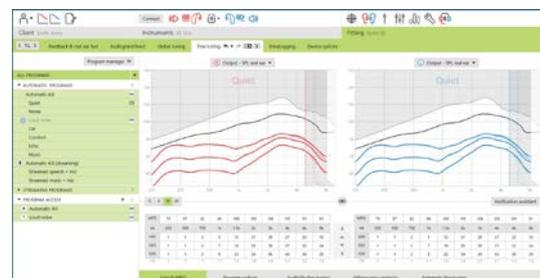
The tabs in the lower part of the screen will offer access to the fitting tools. Each tool has specific modifiers to fine tune the hearing aid.
